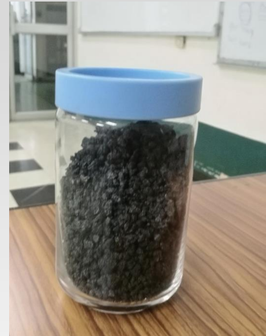
Petroleum coke (90% C)
